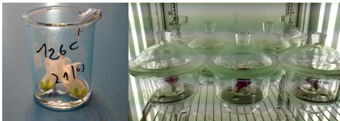
**Figure 4** Left: flowers in a beaker with a Gerstel twister attached. Right: The beakers placed in desiccators in a growth chamber for scent collection.
