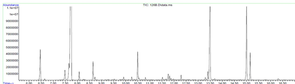
Figure 5 The complete GC spectrum of the emission of line 126B, showing the peaks of the volatiles with the corresponding retention times in minutes.
