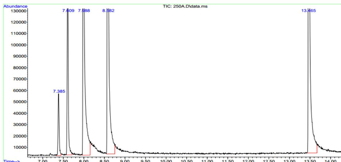
**Figure 8 GC spectrum of the VOCs standards; retention time in minutes**
