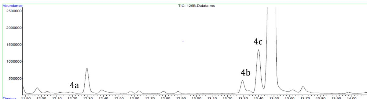
Figure 7 Enlarged interval of line 126B's GC-spectrum ranging from 12 to 14 minutes. The three peaks correspond to methyl cinnamate. 4b and 4c are the same compounds which were separated during analysis due to high concentration.
