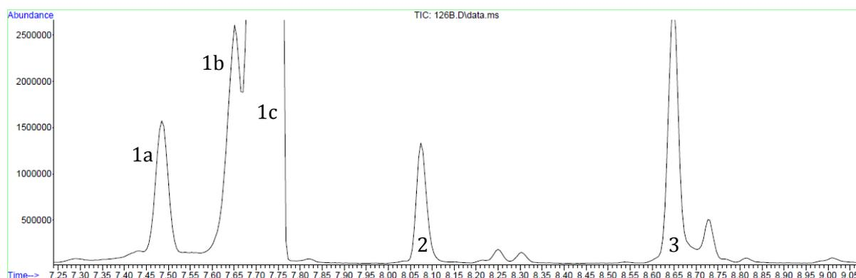
Figure 6 Enlarged interval of line 126B's GC spectrum ranging from 7 to 9 minutes. The peaks numbered by 1, 2 and 3 correspond to ocimene, acetophenone and methyl benzoate respectively.
