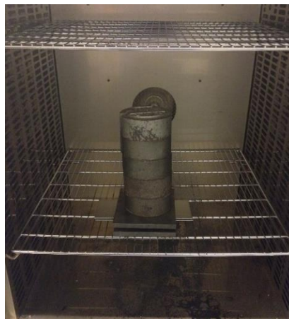
Figure 13: the test setup with the stack of weight acting as pressure
