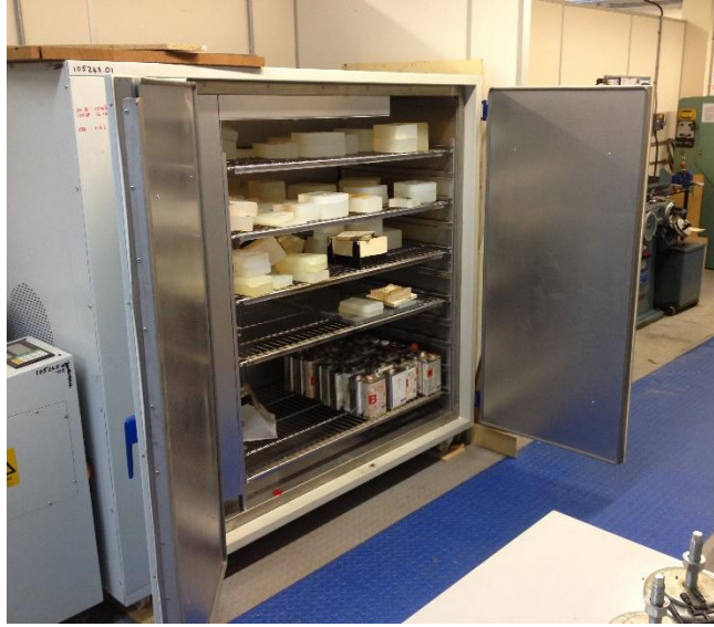
Figure 26: The oven which will be used to perform the annealing
