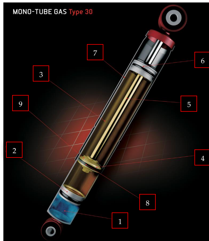
Figure 9: Mono tube shock absorber [16]
