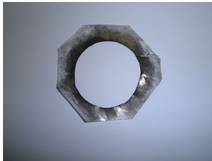
Figure 2.10.: Mask used to paint the electrodes with carbon black. The gap has a diameter of 48 mm .
