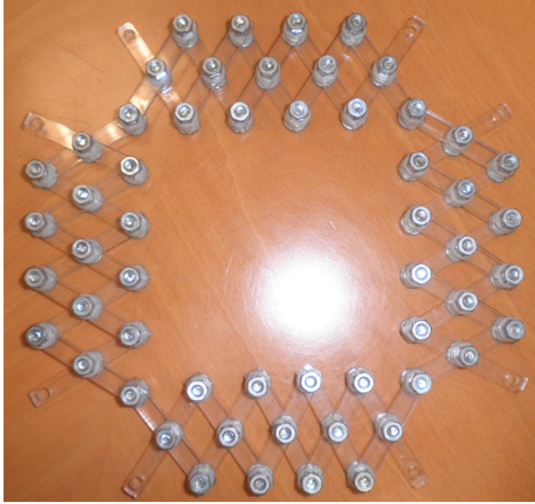
Figure 2.7.: The scissors mechanism made from plexiglass.
