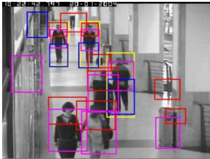
Figure 3: An example of a part-based model technique for human detection. Purple rectangles indicate torsos, red rectangles indicate the head and shoulders, blue rectangles indicate the legs and yellow rectangles indicate full-body detections.
