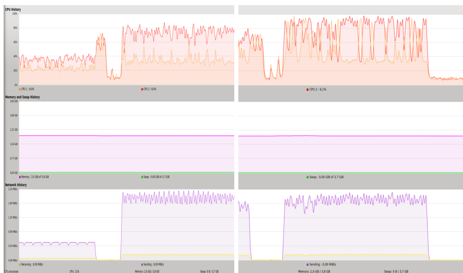
Figure 10.4: CPU and network bandwidth. From left to right: Window size 5 (end of download run), window size 20, window size 60. Note that CPU load increases with the window size, reaching 80% at window size 20 and reaching 100% somewhere between 20 and 60. This means that there is no gain in increasing the window size because of server CPU load.
