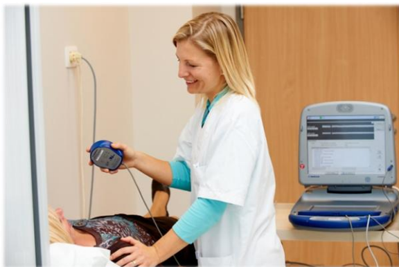
Figure 4: Illustration of a pacemaker programmer. The head will be placed on the site of the implanted pacemaker to allow pacemaker analysis and programming.
