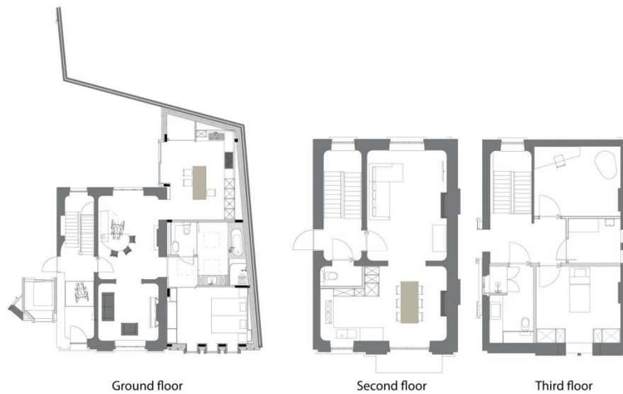
Figure 6. Ground floor (left), 2nd floor (middle) and 3rd floor (right) plan of the housing units
