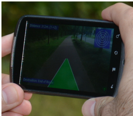
Figure 1: Visual directional cues augment the video feed of the rear camera on the smartphone's display, letting the user perceive both the environment and the guidance at the same time.
