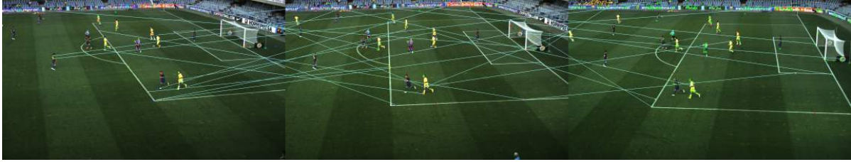
Figure 8: Multicamera feature matches, considered as outliers. These matches were rejected using the angle-based filtering method. There are no false outliers in this example. Only a subset of the multicamera matches are shown.
