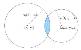
Figure 3: An example of a lens in a space-time prism  $\mathcal{P}(x_i, y_i, t_i, x_{i+1}, y_{i+1}, t_{i+1}, v_i)$ .
