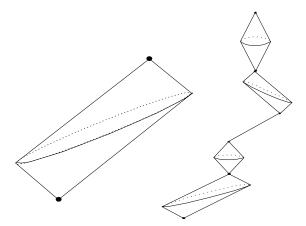
Figure 1: An example of a space-time prism between two consecutive anchor points (left) and a chain of space-time prisms between a sequence of six anchor points with varying speed bounds in between them (right).
