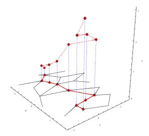
Figure 4: A trajectory on a road network in space-time and its projection on a road network
