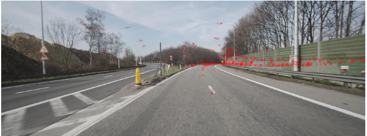
b) Step 2: camera-tracking of 3D reference points
