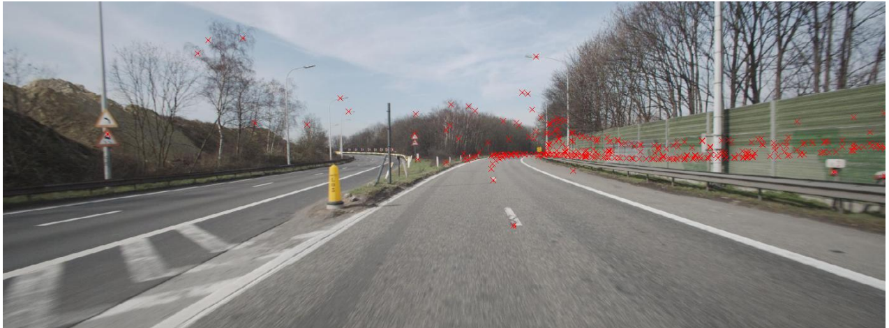
b) Step 2: camera-tracking of 3D reference points
