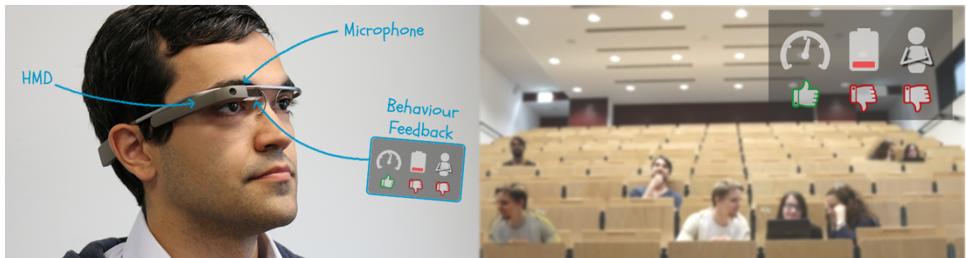
Figure 1. Concept of the Logue system: A user wearing an HMD while giving a public speech (left). Using various sensors and social signal processing techniques (not illustrated), the user receives realtime feedback on his own behaviour superimposed on field of view (right).
