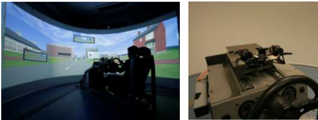
Figure 2. Driving simulator and eye tracking equipment
