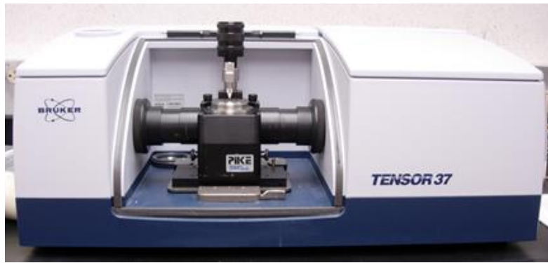
Figure 4.11. Photograph of the FTIR spectrometer device used for identification of functional groups.
