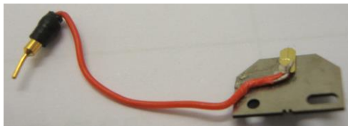
Fig. 6.7. Photograph of the cantilever adaptation to perform conductive measurements on the NX10 AFM.
