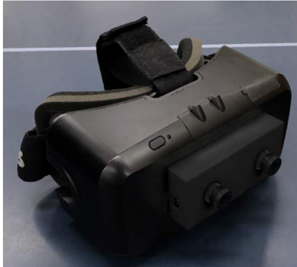
Figure 2.6: Oculus Rift DK2 with an Ovrvision camera attached - Example of a video see-through display
