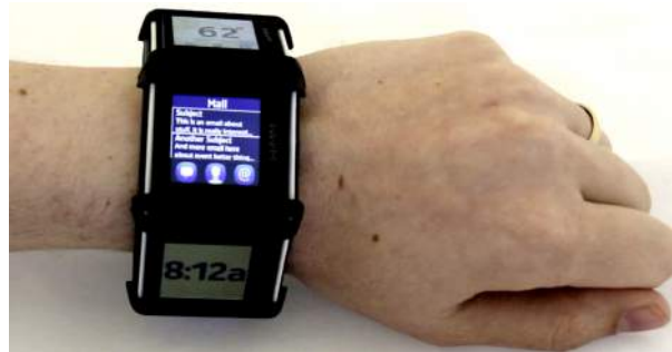
Figure 6.4: Facet - Example of a multi-display smartwatch [24]
