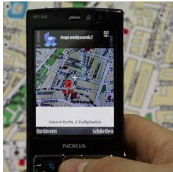
(b) Example of an augmented magic lens used to show additional information based on POI (parking spots) [34]
