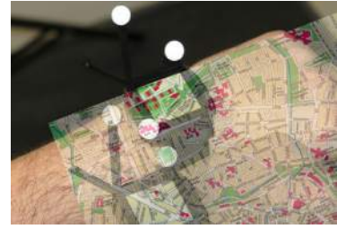
(c) A dynamic peephole display implemented on a smartwatch using a wireless tracking system [17]
