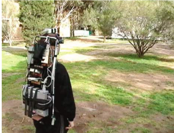
Figure 2.3: Example of an AR application, requiring hardware to be worn as a backpack [2]
