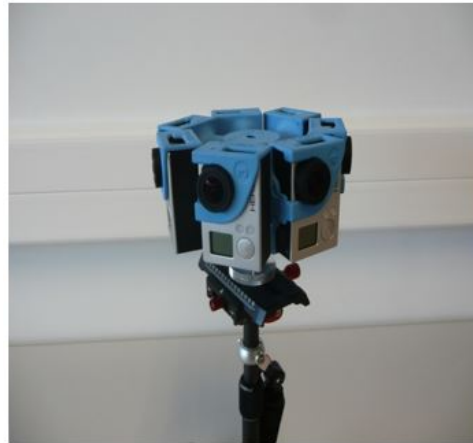
Figure 4.3: 360 degree ODV camera stand involving 7 GoPro cameras
