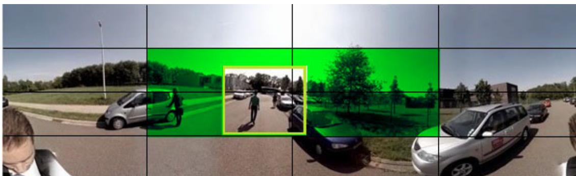
Figure 4.7: ODV full frame divided into a 4x4 grid with indication of the current viewport and un-visible parts
