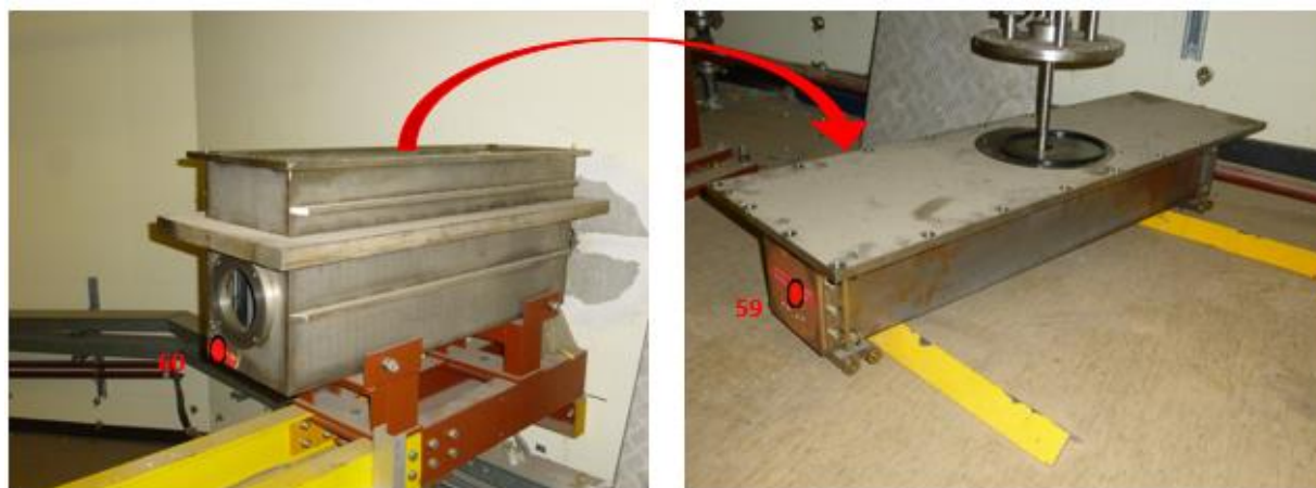
Figure 62 - Box and solid iron structure to stop the beam during emergency
