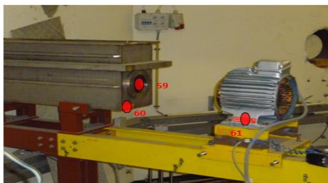
Figure 53 - Sample locations in cast-iron focus lens and box to stop the beam during emergency
