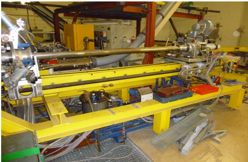
Figure 67 - Structure on which the internal target was mounted
