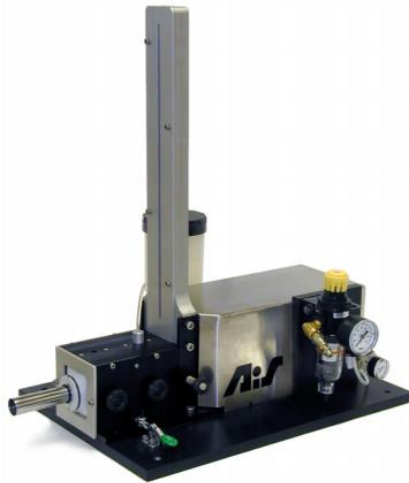
Figuur 36: O-ring montage machine AIS [12]
