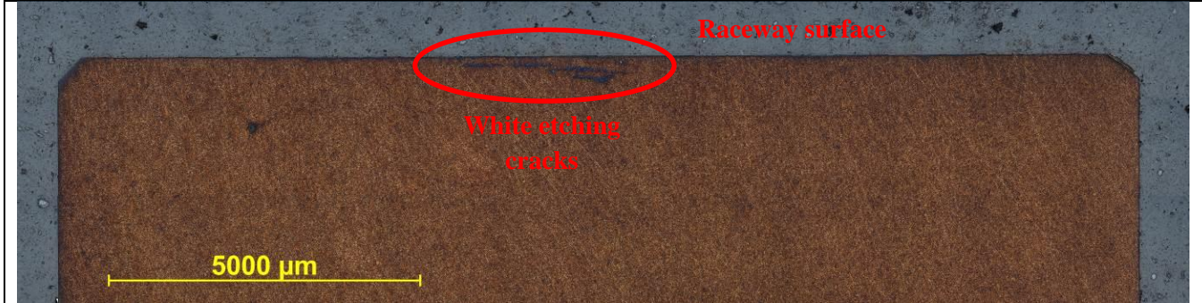
Figure 1 (4:1) Nital etched 3% Raceway surface overview with white etching cracks
