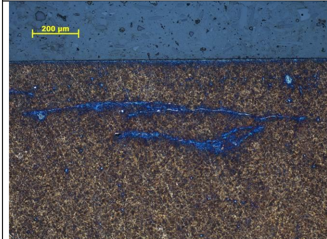
Figure 1 (100:1) Nital etched 3% White etching cracks
