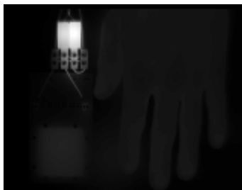
Figure 5.6: An element of the IR image stream of the meander resistor, as provided by the FLIR E40 IR camera.
