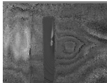
Figure 5.15: The phase image of the CFRP substrate with defect subjected to a lock-in IR thermography experiment.
