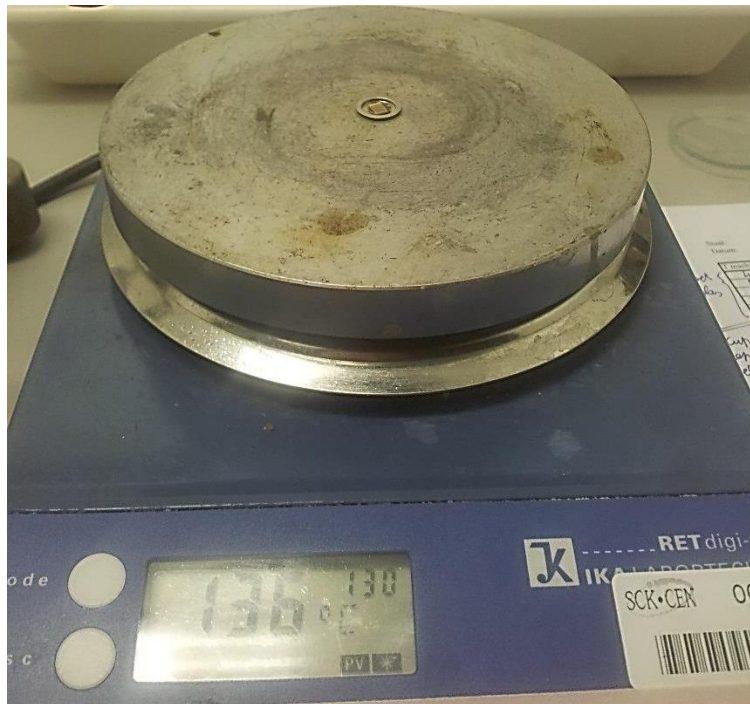
Figure 4-53: Simulation of the Risø heating plate by a controllable heating plate (RET digi-visc from IKA Labortechnik, SCK serial number 002484)
