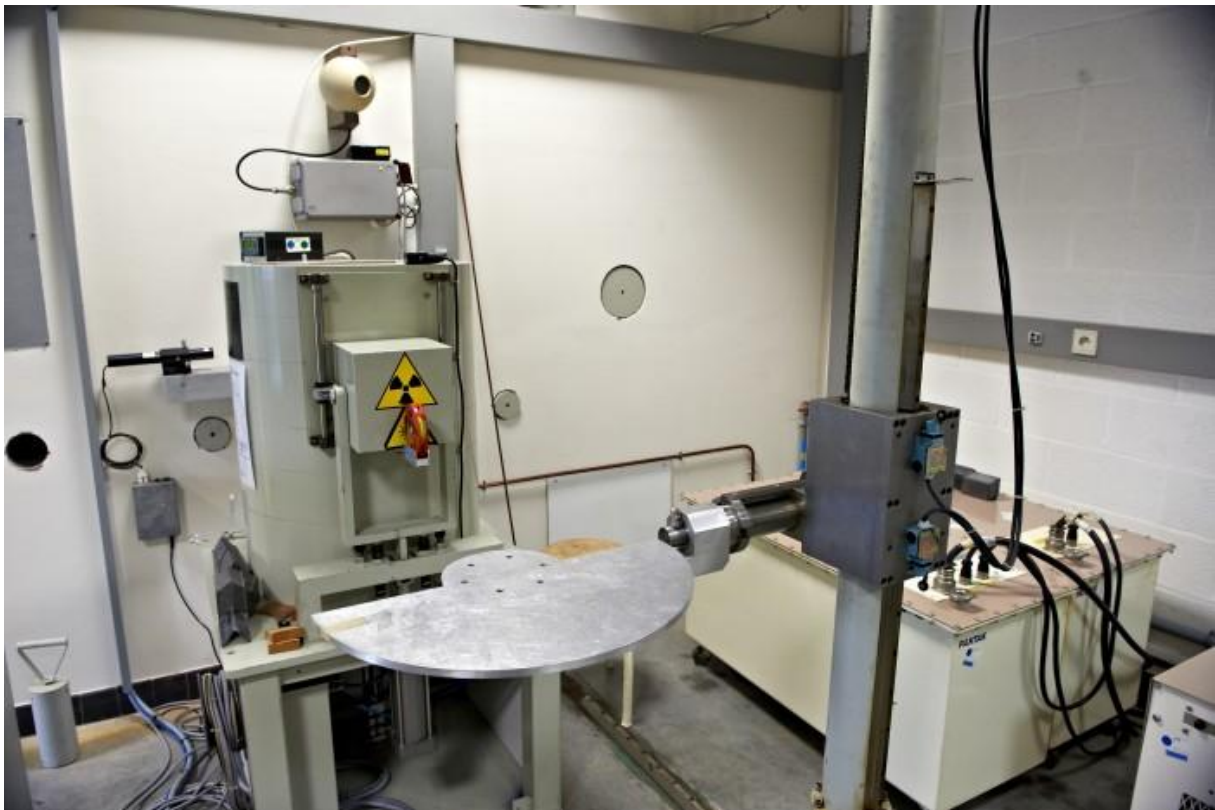
Figure 3-1: The horizontal set-up with 3 sources of ^{60}\text{Co} and 3 sources of ^{137}\text{Cs} [29]
