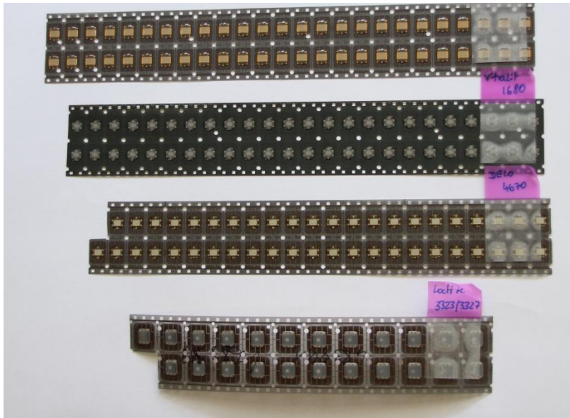
Figure 3-21: Morpho SIM card modules covered in epoxy (back side); from top to bottom: Delo 689-4670 ; Vitralit 1680 ; Delo 4670 ; Loctite 3323-3327
