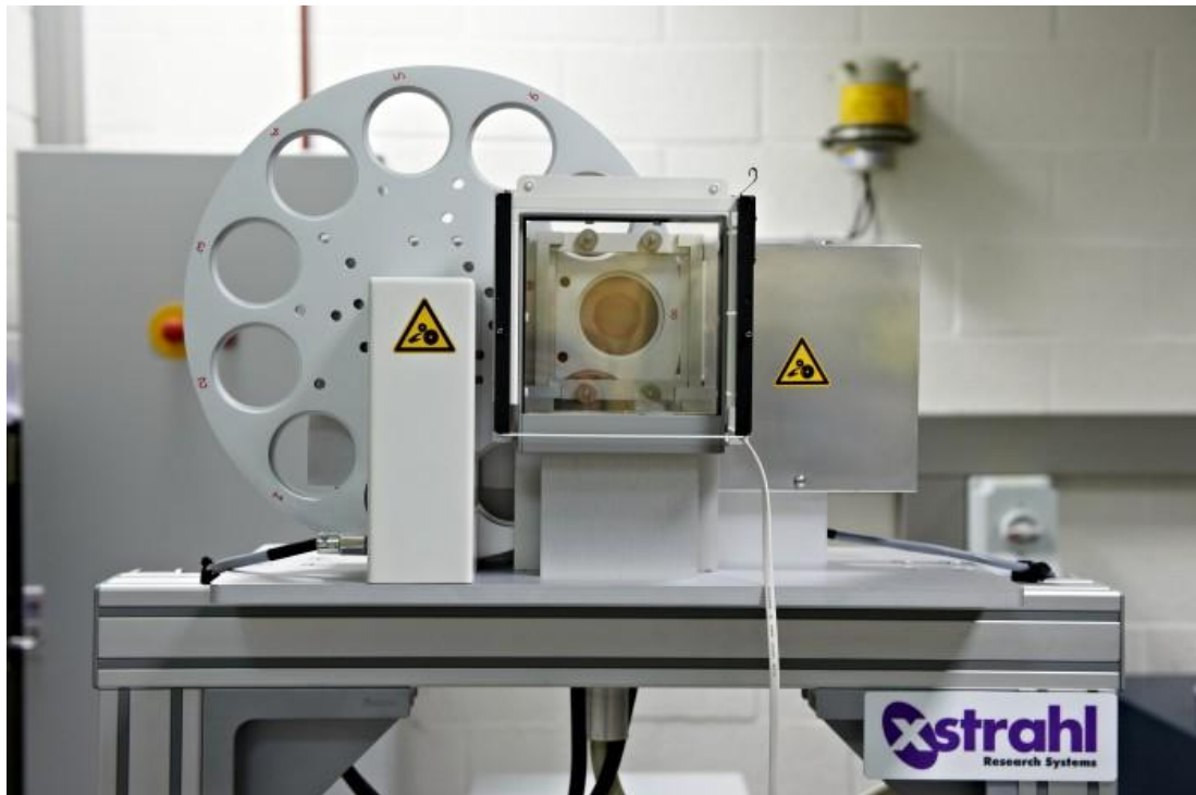
Figure 3-3: X-ray generator with automatic filter wheel [29]
