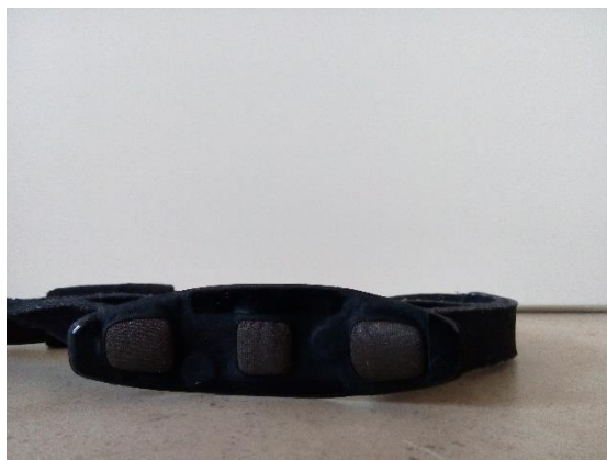
Figure 7: Electrodes made of silver coated fabric
