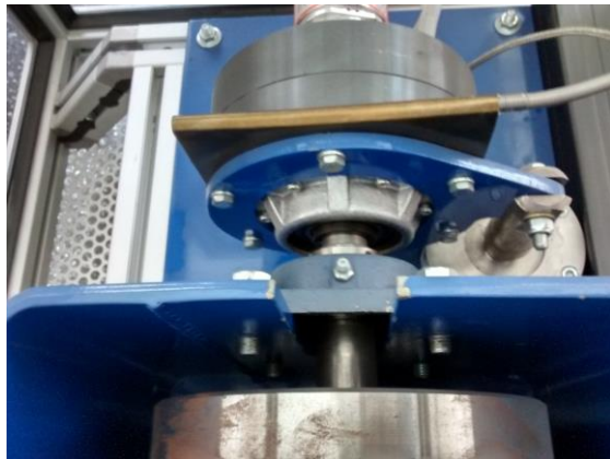
Figure 26 Left: Brake with load cell. Right: Occurring forces
