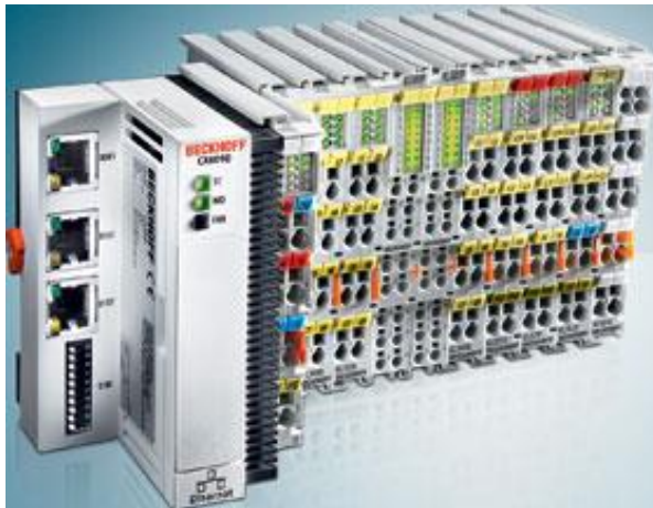
Figure 1 A Beckhoff PLC with the controller module and I/O modules [1].
