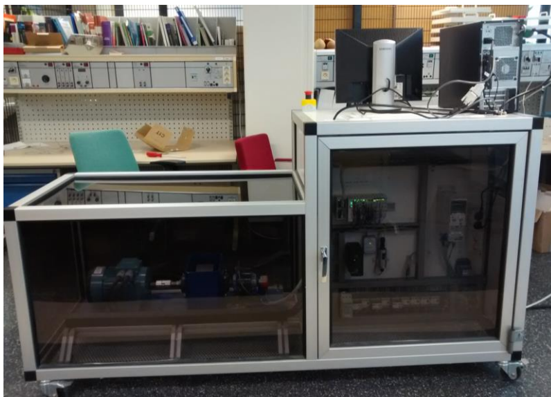
Figure 65 Completed motor test unit
