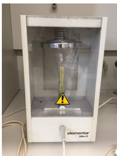
Figure 19: Installation of the Schöniger flask in the combustion device (Mikro K, Elementar)
