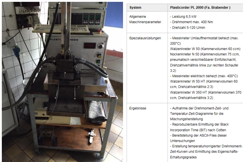
Figure 16: Plasticorder PL 2000, Brabender for mixing of NR and SBR
