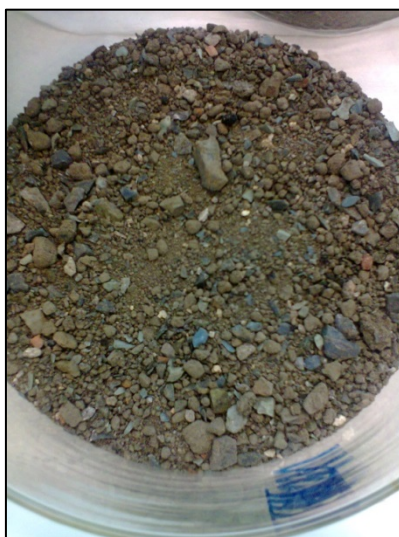
Figure 31: Ungrinded ferromolybdenum hot spot
