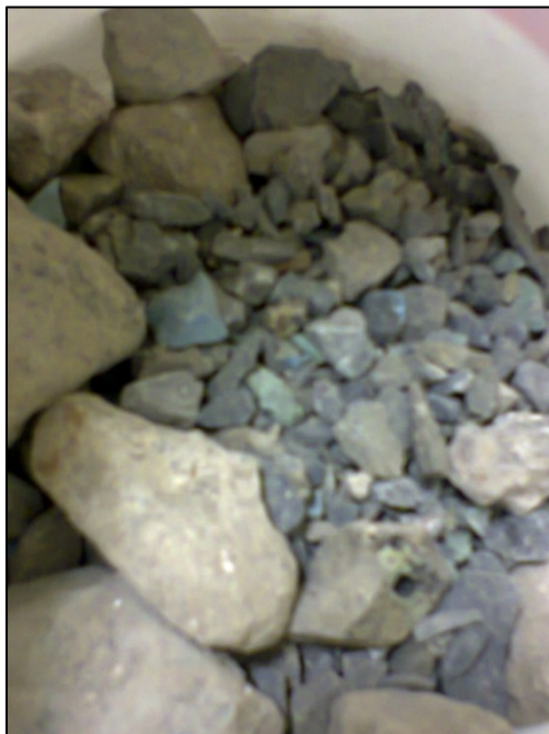
Figure 29: Ungrinded ferromolybdenum slag
