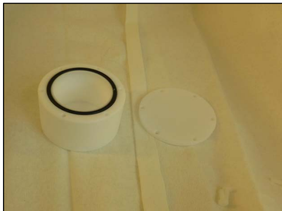
Figure 28: Radon tight PTFE container
