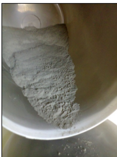
Figure 30: Grinded ferromolybdenum slag
