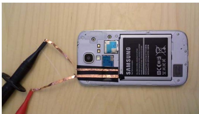
Figure 29. Bypassing the battery of the phone [25]
