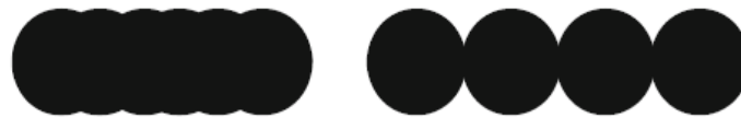
Figure 22 : Schematic representation of the effect of higher point distance on the roughness
