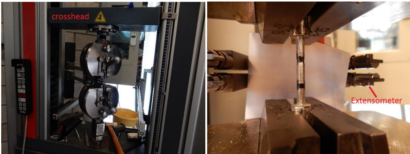
Figure 48 : Left: Tensile test bench Zwick Z050, Right: Example of how a horizontal piece is clamped in the machine
