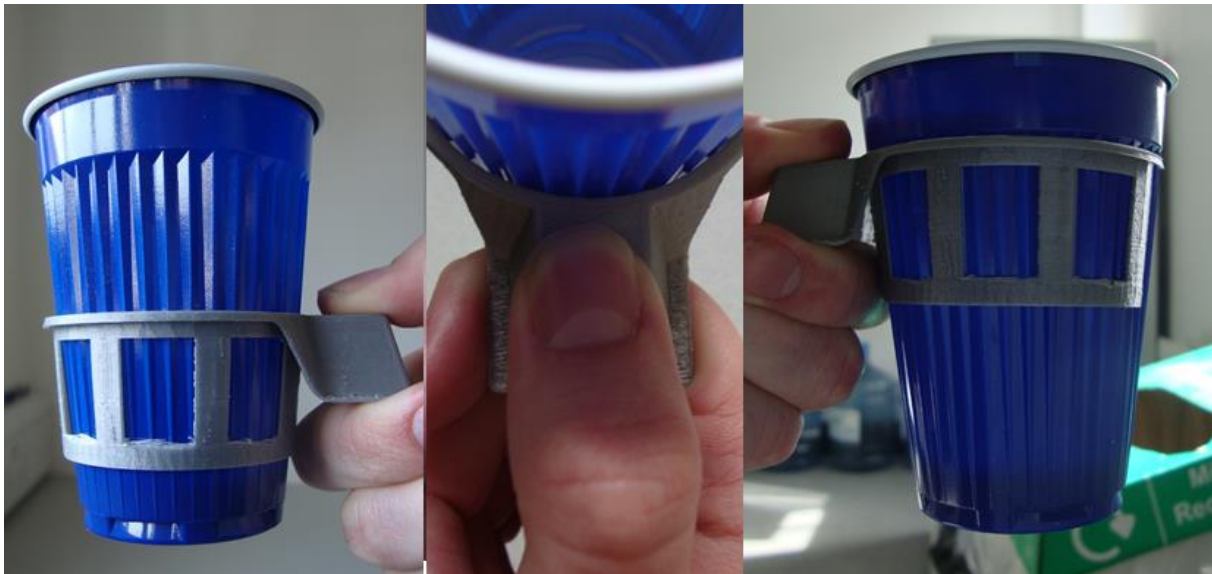
Figure 55 : Ergonomic test of the first product; left: side view with empty cup, middle: top view with empty cup, right: side view with full cup
