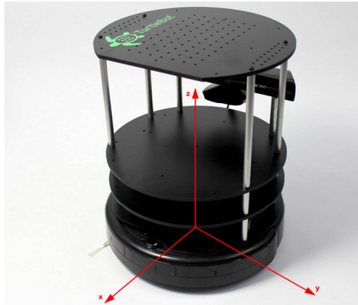
Figure 42: The coordinate-system of the Turtlebot [55].
