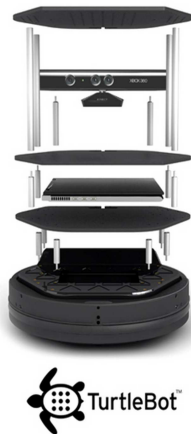
Figure 23: The Mechanical Design of the Turtlebot [20].
