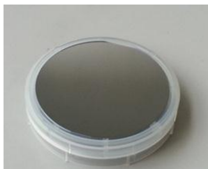
Figure 2: The surface of cleaned silicon wafer
