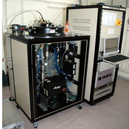
Figure 3: ASTeX reactor for BNCD growth
