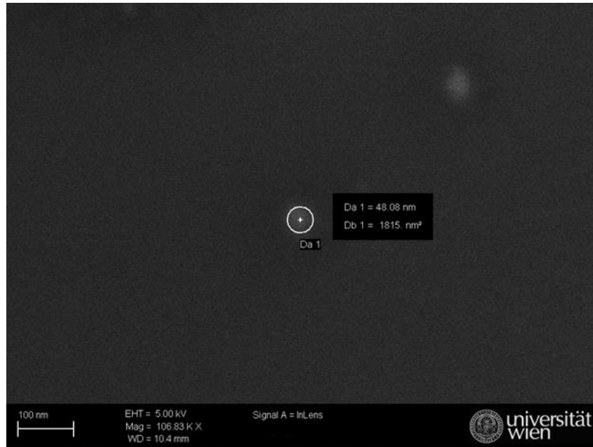
Figure 3.3. SEM picture of a single silver sulphide nanoparticle.
