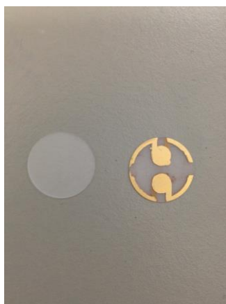
Figure 2.1. Pictures of blank quartz crystal (left) and gold-printed quartz crystal (right).
