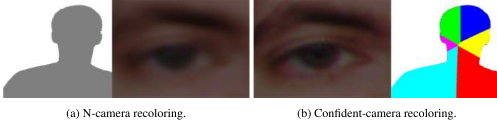
Figure 7.9: The recoloring module recolors the refined depth map to produce the final interpolated image. (a) N-camera recoloring equally blends all N input cameras. (b) Confident-camera recoloring selects a single input camera that is closest in angle to the virtual camera, determined using the color-coded index map in which each color represents another input camera.
