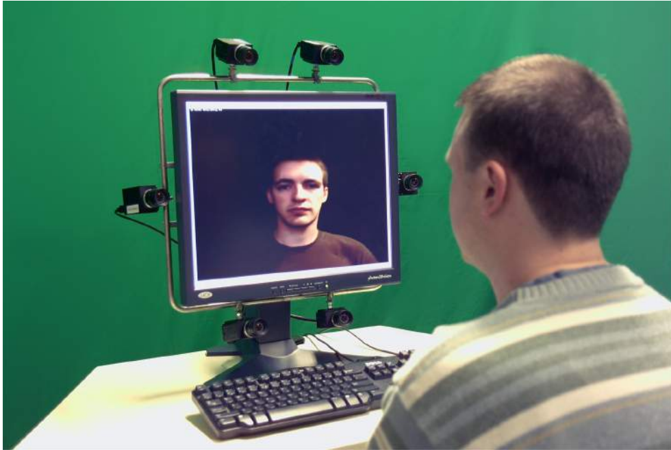
Figure 7.2: Our fully functional end-to-end prototype for close-up one-to-one eye gaze corrected video conferencing. Six cameras are mounted on a custom-made lightweight metal frame closely surrounding the screen: two above, two below and one to each side.
