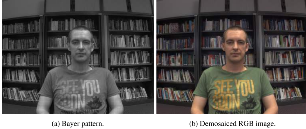
Figure 2.12: (a) A one-channel RGGB Bayer pattern must be (b) demosaiced into an RGB image.
