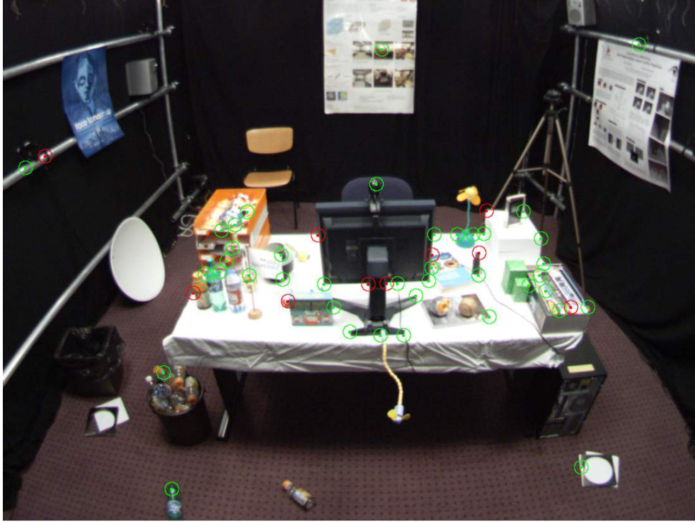
Figure 3.3: Given a set of detected features with an established rank-order, we can extract two subsets with high (red markers) and low (green markers) intra-element distances. We label them the primary and secondary hotspots respectively.
