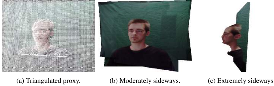
Figure 7.16: Unstructured lumigraph rendering from non eye gaze corrected viewpoints. The refined depth map has been triangulated into (a) a geometry proxy, which has then been rendered from (b) a moderately deviating viewpoint and (c) an extremely deviating viewpoint. In particular the latter shows that the refined depth map approximates the true shape of the face well.
