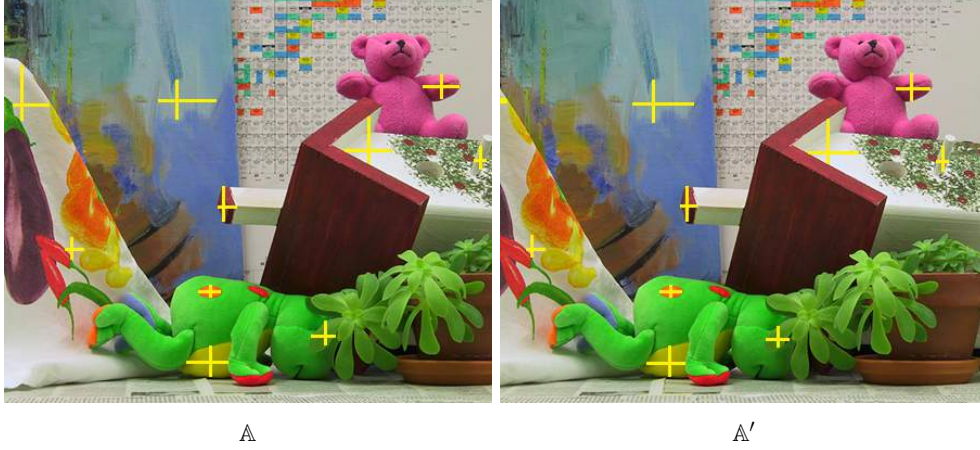
Figure 5.4: Some left ( \mathbb{A} ) and right ( \mathbb{A}' ) axis quadruplets from Equation 5.1, drawn as yellow crosses of their horizontal and vertical axes.
