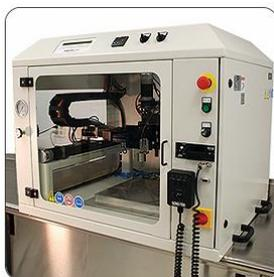
*Figure III-22: Photograph of an ExactaCoat Ultrasonic Coating system of Sono-Tek Corporation in combination with an AccuMist Precision Ultrasonic Spray Nozzle.[20]*
