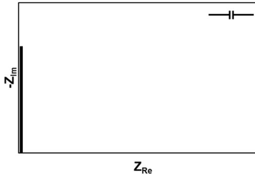
Figure I-33: Nyquist plot for an ideal capacitor. As an inset the symbol of an ideal capacitor is shown.
