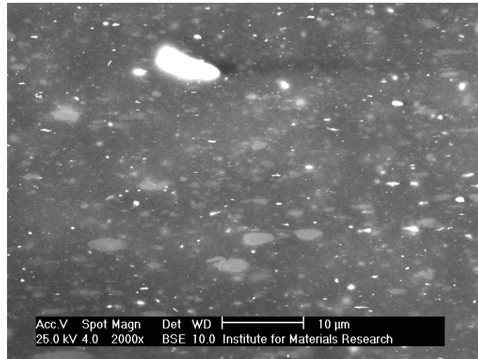
Figure 3.5: SEM cross-section image of a dense PTMSP-silica (10 wt.%) membrane.
