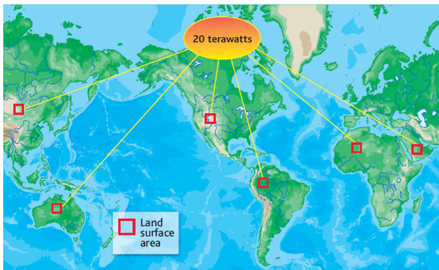
Figure 1. The land surface area needed to generate 20 TWh with 10% efficient solar cells. 2
