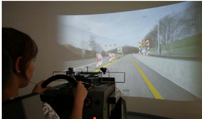
Fig. 3. Traffic Sign Simulator mock-up with eyetracking system.
