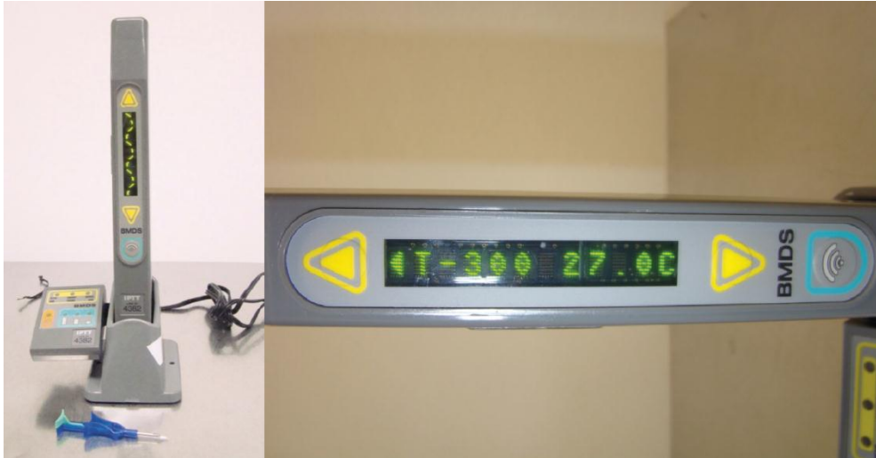
Fig. III.2. A validated probe thermometer (Plexx thermometer) with implantable transponders for reading the peripheral body temperature without disturbing the animals.
