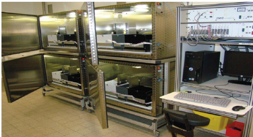
Fig. III.6. The CPP apparatus is placed in soundproof box, and connected with the IT system.
