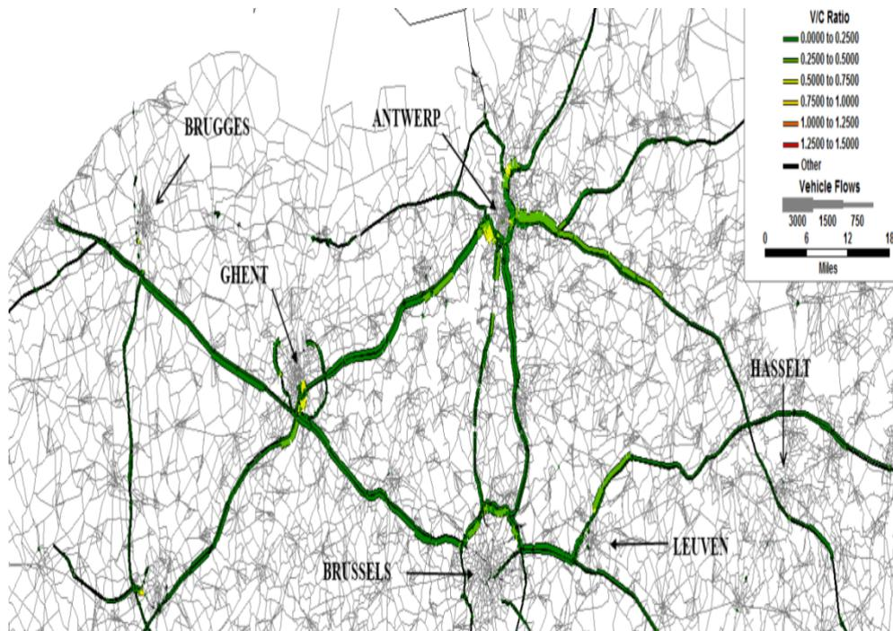
Figure 4.5 Mean link traffic flows in highways for work/school trips between 7 am and 8 am from DUE assignment and PG predictions based on the mean link flow vector from method 1.
