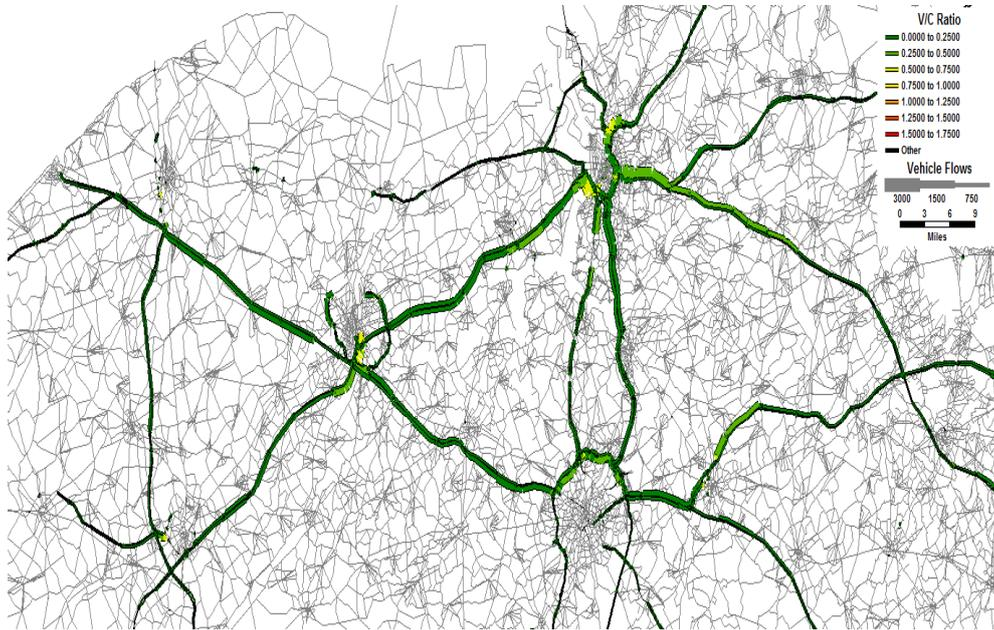
Figure 4.10 Mean link traffic flows in highways for work/school trips between 7 am and 8 am from DUE assignment and PG predictions based on the mean link flow vector from method 2.
