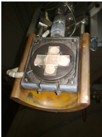
Figure 3.4: The substrate holder of the sputter system. The front part of the radiation shield is removed for better visibility. The heat shield and steel box (radiation shield) are clearly visible. One (0002) sapphire ( \text{Al}_2\text{O}_3 ) substrate and four additional sapphire platelets to ensure homogeneous heat spread, are glued directly on top of the inox heater disk.
