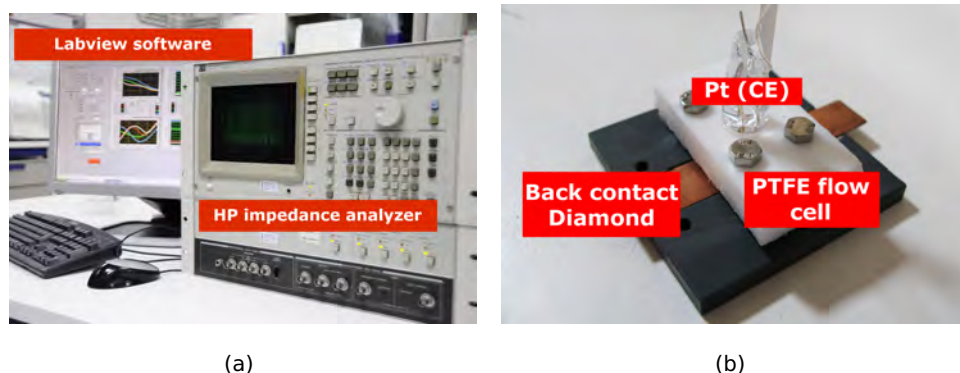
Figure 4.9: Instrumentation used for the time resolved impedance measurements with in (a) the HP4194A impedance analyzer with home-made software on the Labview platform and in (b) a home made single channel flow cell with Pt counter electrode.
