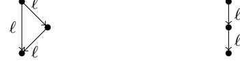
Figure 4. Two simple graphs. Only on the graph to the left, the navigational expression \ell^2 \cap \ell evaluates to true .
