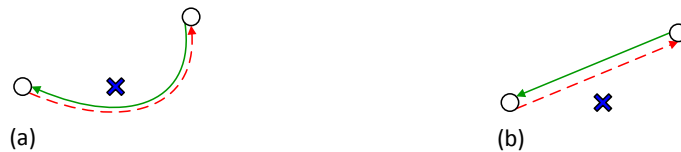
Fig. 1: (a) Situation with geometry: bus stop is connected to the (correct) solid green link. (b) Situation where the geometry is replaced by a straight line segment: bus stop is connected to the (wrong) dashed red link.
