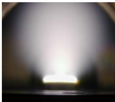
Figure 2.4: Photograph of the ASTeX-type reactor present at IMO (left); picture of the plasma ball during the diamond growth process with reactant gasses: 0.05% \text{CH}_4/\text{H}_2 and 500ppm \text{PH}_3/\text{CH}_4 (right).
