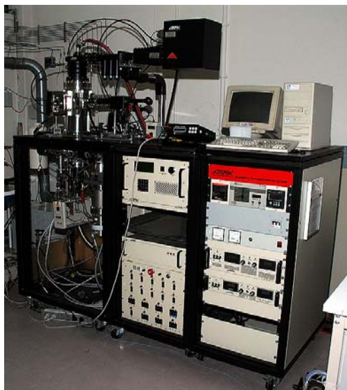
Figure 2.4: Photograph of the ASTeX-type reactor present at IMO (left); picture of the plasma ball during the diamond growth process with reactant gasses: 0.05% \text{CH}_4/\text{H}_2 and 500ppm \text{PH}_3/\text{CH}_4 (right).
