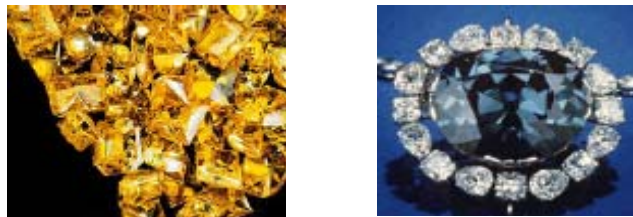
Figure 1.6: The difference in colour caused by impurities in the diamond lattice: image of nitrogen containing HPHT diamond crystals (left) and a picture of natural boron-doped diamond, the famous Hope diamond (right) (Schreck 2008).
