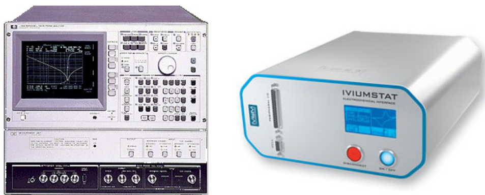
Figure 2-20: HP 4194A Impedance/gain phase analyzer (right) and an Iviumstat electrochemical analyzer (left).
