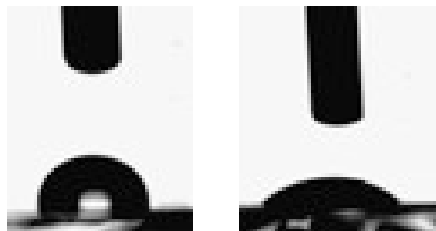
Figure 2-11: Contact angle of a hydrophobic (left) and a hydrophilic (right) surface.
