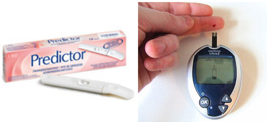
Figure 1-1: The home pregnancy test (left) and the glucose sensor for diabetes patients [OneTouch® Ultra® 2 from LifeScan] (right) are both examples of successful, commercially available biosensor.
