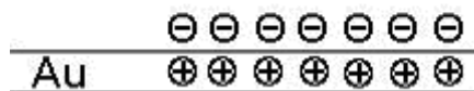
Figure 2-16: Schematic representation of the formation of a double layer capacity at the electrode, according to the Helmholtz model.
