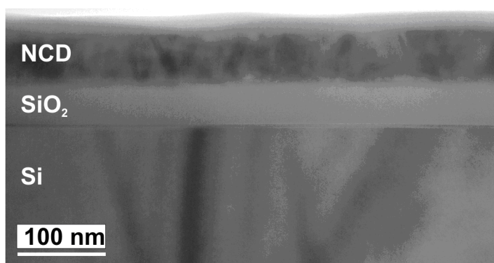
Figure 6.6. EDIS structure cross section (SEM image).
