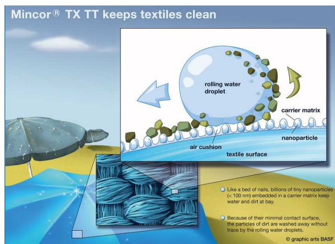
Figure 1.11: Schematic representation of the Mincor TX coating, developed by BASF. The coating exploits the lotus-effect in order to obtain self-cleaning textiles ( www.BASF.com ).
