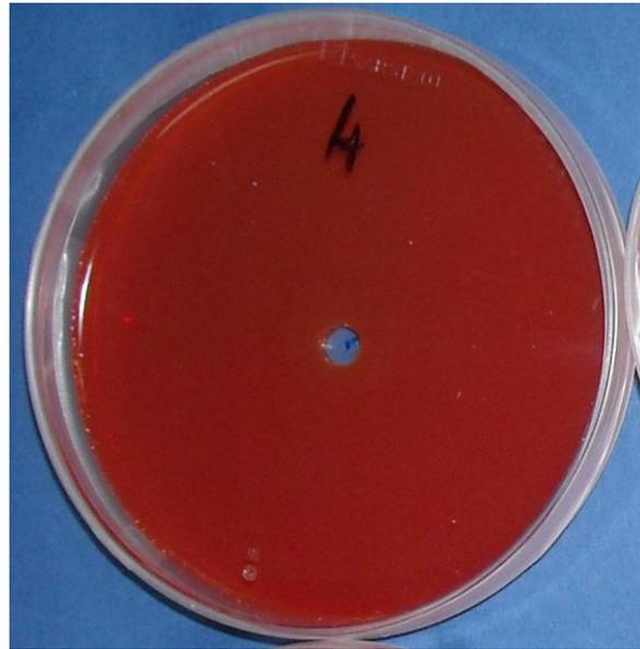
Fig. 17 Lipase activity test on strain n. 4.
