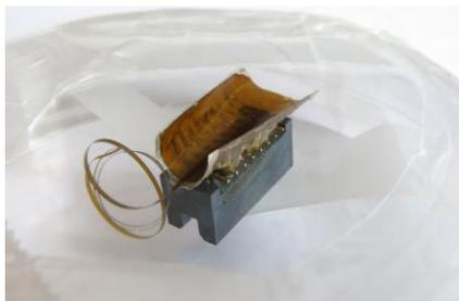
Figure 4-23. Conductive tape peeling off from the electrode and the connector due to curling of the electrode.
