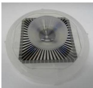
Figure 3-15. Flexible reusable cell culture silicone chamber (Greiner BioOne) was attached to MEA, creating a bath chamber required for electrochemical impedance measurement under PBS.
