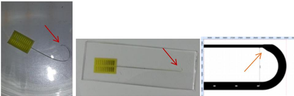
Figure 4-20. Weak attachment of needle to the electrode which caused losing the needle in releasing process. The fragile attachment of the needle in the design is shown.
