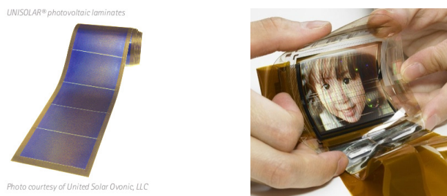
Figure 3. OPV (left), OLED display (right).
