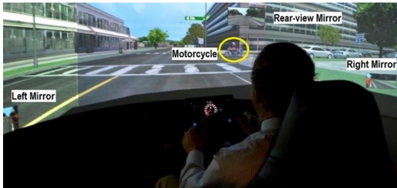
Figure 31: Simulator Displaying a Road Hazard (Motorcyclist Emerging from Behind Traffic) Requiring a Defensive Maneuver. Rear View Mirrors are Located to the Left and Right.
