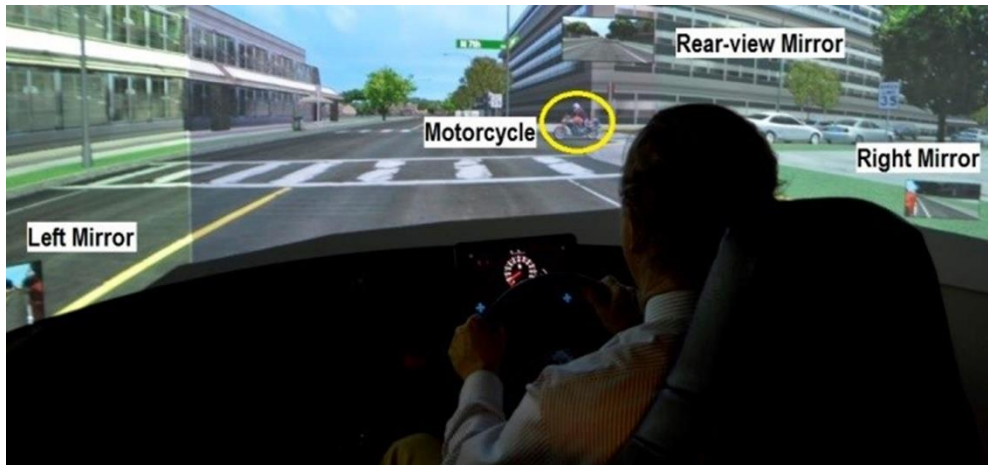
Figure 28: Simulator Displaying a Road Hazard (Motorcyclist Emerging from Behind Traffic) Requiring a Defensive Maneuver.
